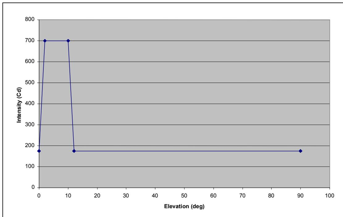
**Figure 3** Vertical Beam Characteristics for Current Operating Minima (1400m minimum meteorological visibility)
