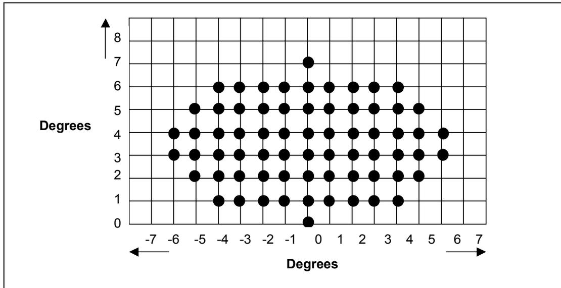
**Figure 1** Typical Intensity Distribution Measurement Diagram
