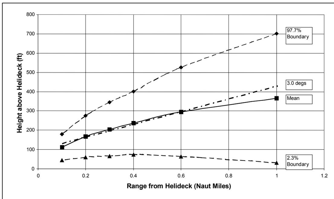
**Figure 1** In-Service Data on Vertical Approach Profiles
